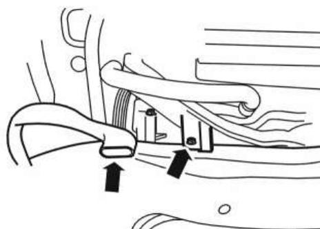
Remove the screw, 1 pc. for the cable channel and loosen the cable channel from the sub-frame.
