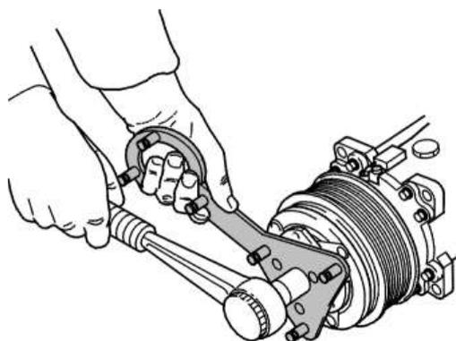
Loosen the screw, 1 pc., for the drive plate using a counterhold: 999 5596 .
