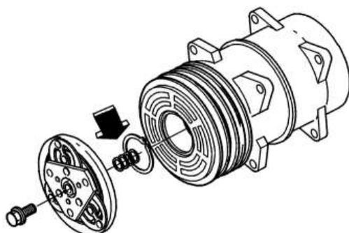
Loosen the drive plate using a puller: 999 5597 .
