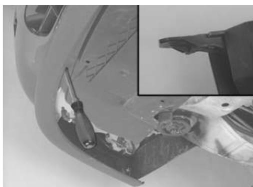
Remove the screws, 2 pcs., for the front protective cover.
